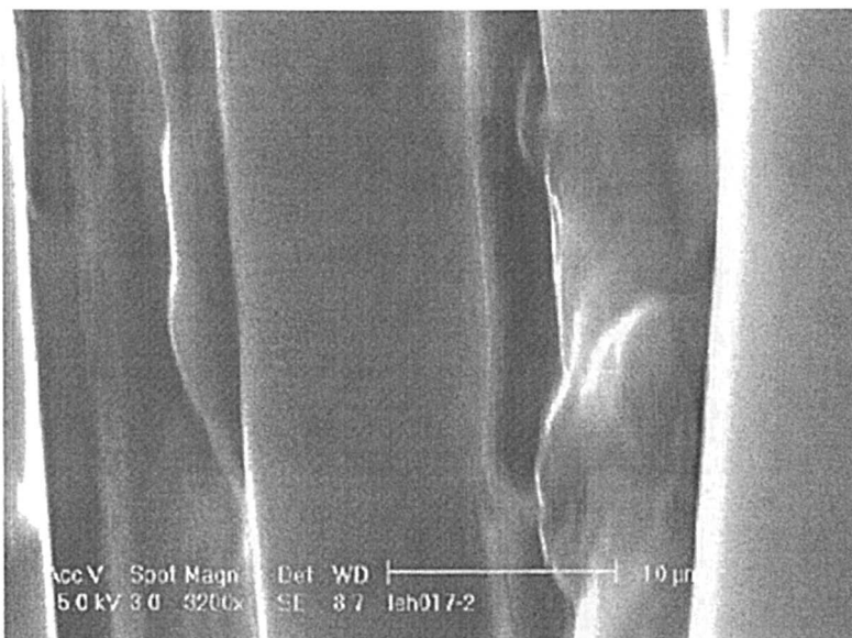
Figure 6. SEM micrograph of poly 1-[(2-vinylxy)ethoxy]ethyl acetate triethoxysilane coated E glass fibers after the complete washing process.
